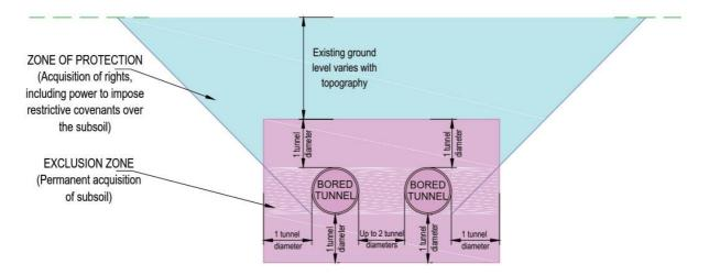
**Figure 1** - Illustrative cross-section showing land acquisition through the tunnel section. Pink signifies permanent acquisition of land, blue signifies permanent acquisition of rights only (including rights to impose restrictive covenants for the protection of the tunnel).
